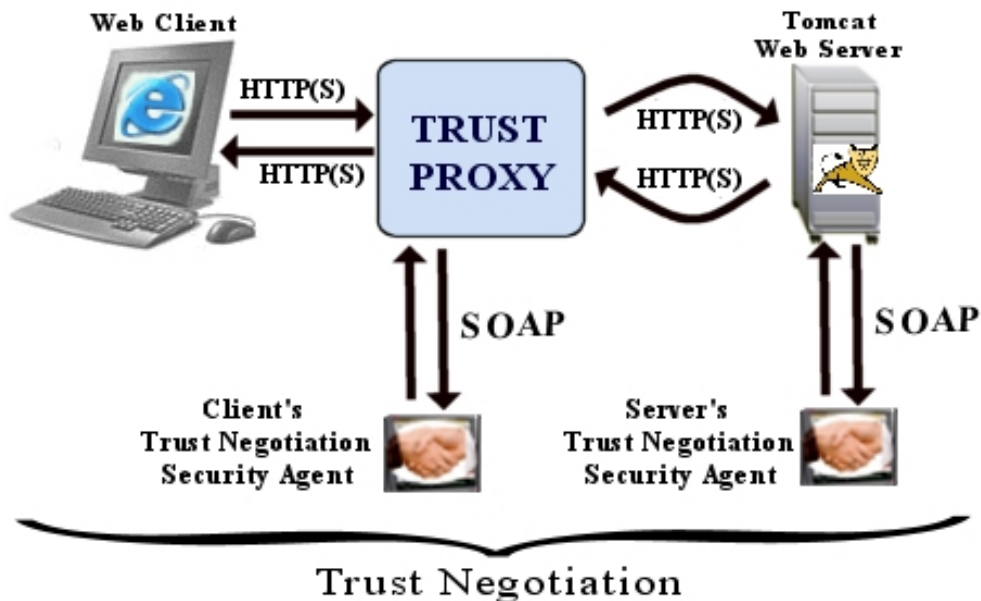
Figure 12 – The TrustBuilder Implementation Architecture. The web client’s HTTP requests are handled through a trust proxy supporting trust negotiation. SOAP is used to communicate from the application layers to the independent security agents, and all other messages between the client and the server are over HTTP(S).
